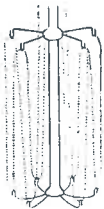
The supporting wires are light and act as springs to absorb shock.
