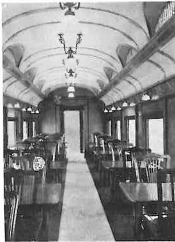
Mazda lamps and Holophane reflectors attached to special fittings in dining car.
